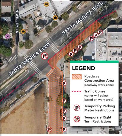
Images for illustration purposes only. Example of how traffic will shift depending on the work zone. Not an accurate traffic control plan.
